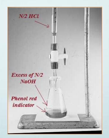
As in other quantitative determination involving boiling with a standard alkali, cooling and back titrating the excess, it's necessary to carry out a blank experiment without the aspirin In order to:
